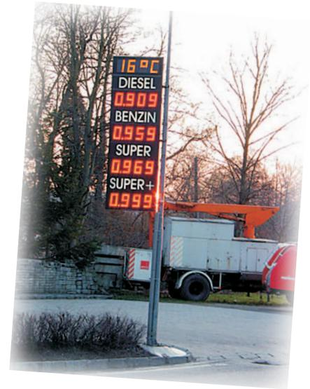
Basically our displays are realized with about 3000mcd ultrabright AlInGaP II leds for absolute good readable also under direct sunlight. The brightness intensity will be automatically dimmed in 256 steps according to the daylight level.
